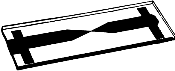
FIG. 43.—SLIDE WITH GOLD-LEAF ELECTRODES.
